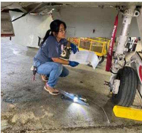
Brenda Gratz A&P, utilizing the checklist and lubrication chart on the left main landing gear the T28 Bravo
