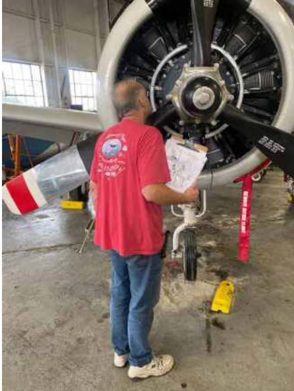
Andrew Gratz A&P checking the reassembly of the Cowl on the T28 Bravo post lubrication and inspection
