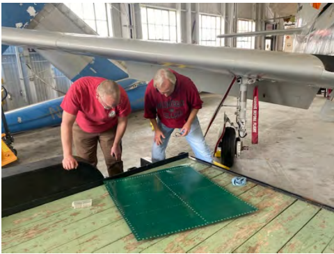
Frank Fry and Dave Biloz work on replacing the rivets on the panel for the C45.
