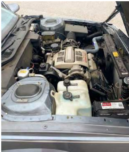
Left: 3.8L V6 with the automatic 4-speed transmission (overdrive) with soft ride suspension
